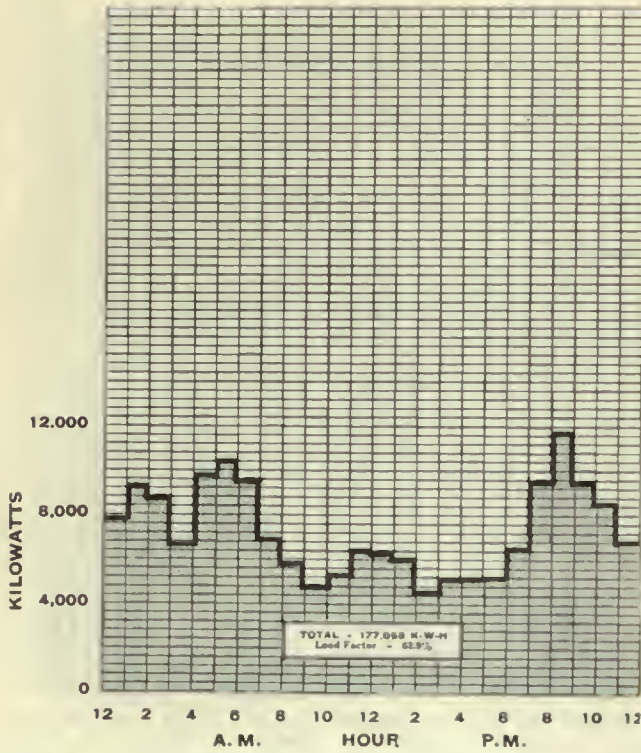
FIG. 600. ENERGY CHART. Kilowatt-Hours at the Pantograph for the Average October Day for 11,000-Volt A. C. Operation, Road Freight Service.
